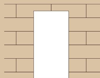
Arrangement of boards at openings
