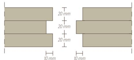
Tongue-and-groove ensures a good bond and a level substrate for subsequent plastering.
