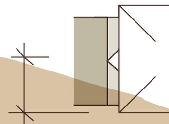
approx. 8 cm between the beam's outer edge and the middle of the triangular batten
