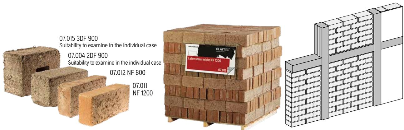
Lightweight mould-made clay block of application class Ia (= approved for timber-frame masonry work) in format NF. The composition and manufacturing technique make it very resistant to moisture and frost. The historical normal format (NF) lies well in the hand, the size is just right for timber-frame construction. The 1200 NF clay block can be knocked and cut into shape very easily. Lightweight clay masonry mortar is an ideal mortar for plastering with coarse lime basecoat render with hair.
