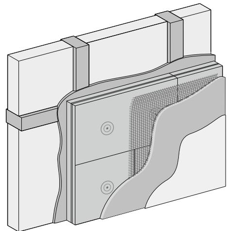
Wood fibre insulation board for interior insulation of timber-frame houses and all other historical buildings. CLAYTEC HFD interior insulation boards are glued locally in a clay plaster levelling course or fixed with clay adhesive and reinforcing mortar. The soft boards decouple deformations in the construction from the interior plaster. They are inexpensive and suitable for many types of wall.
